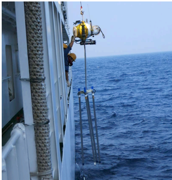
Fig. 3-6 Recovery of an OBEM in this cruise
