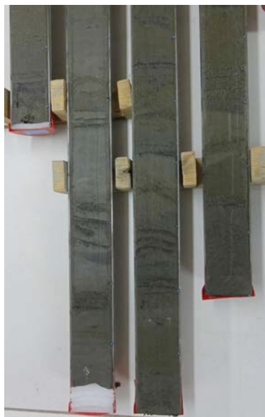
Fig.4.1: Frequent occurrence of turbidite layers observed in PC21 (core diameter = ca. 74mm)
