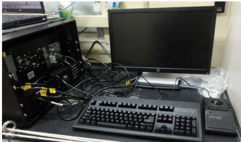
Fig. 4.2.2 Deck unit of a sub bottom profiler system in the control room.
