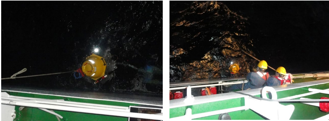
Fig 5.2.2 Recovery operation of the OBEM at starboard of the vessel.
