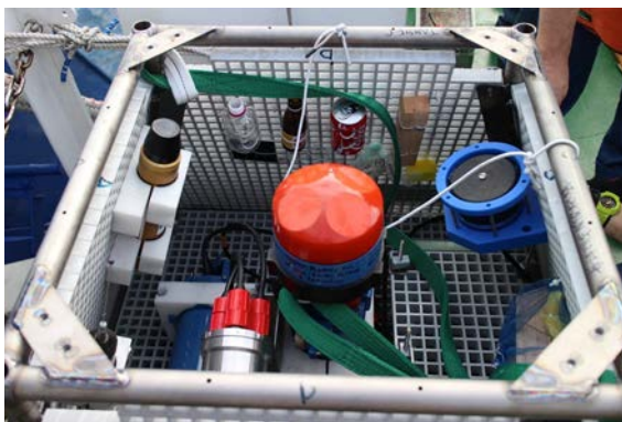
Fig. 7.1.2. Photo taken from the top part of the lander. Green belt was connected with the transponder of the mooring system with a titanium ring.
