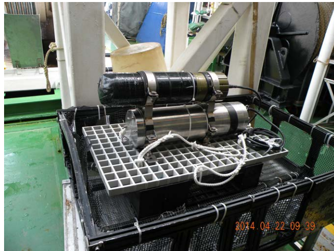
Fig. 4-2 The automatic gamma ray spectrometry system developed for the present study.
