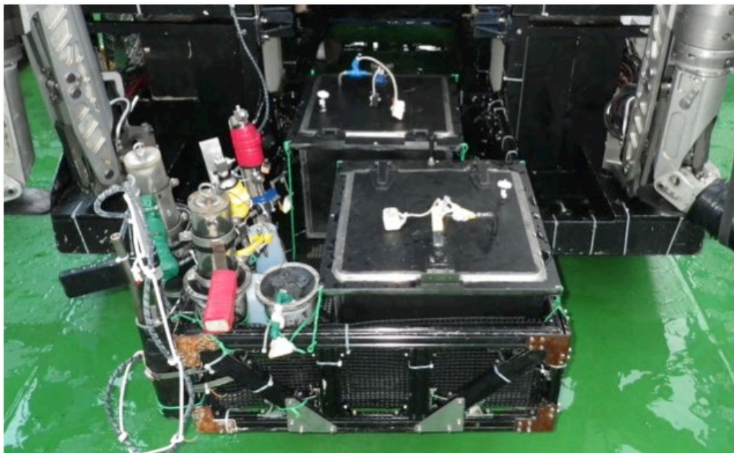
Figure 7 On-line thermometer, Niskin water sampler (x2), Sampling box for in situ incubator (x2), DO meter, M-type sediment sampler (x2), Vacuum water sampler (x2)
