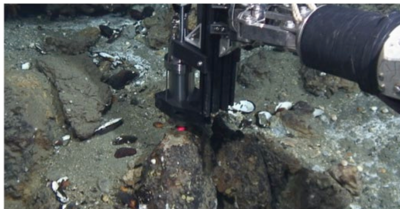
Figure 5 Guide laser (red spot) used to align and focus ChemiCam's main pulsed laser, which generates a plasma from the target once a second.
