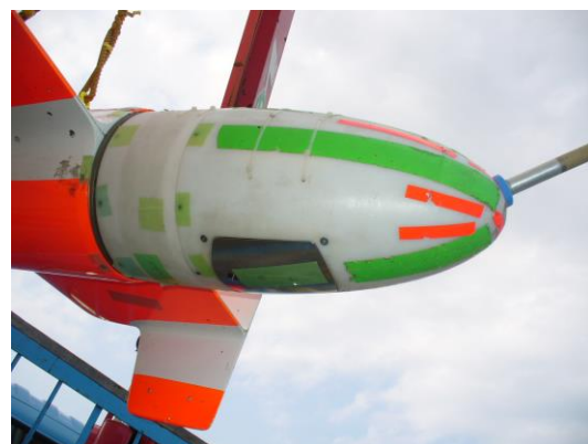
Fig. 6 Ballast on the vehicle
