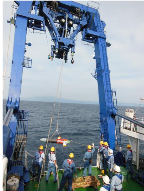
Fig. 7 Photo of the vehicle being raised up by the A-frame
