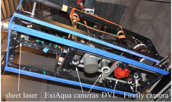
Fig. 1: SeaXerocks mapping system mounted on payload skid.
