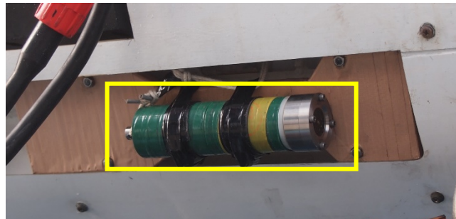
Figure 5: Turbidity meter on the starboard bow of AUV Yumeiruka hull.
