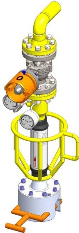
Fig. 3-6 Simplified flow meter with pressure and temperature gauges with a sensor logger.
