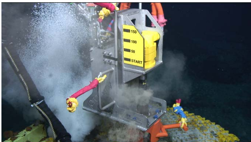
Fig. 3-14 Removing scale within the steel pipe by hydraulic power drill.
