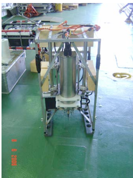
Fig. 1 Profiler module for in situ high-resolution microprofile measurements of O 2 , pH, H 2 S and temperature.
