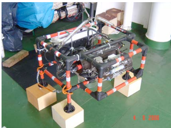
Fig. 2 Benthic chamber module for in situ total exchange rate measurements.
