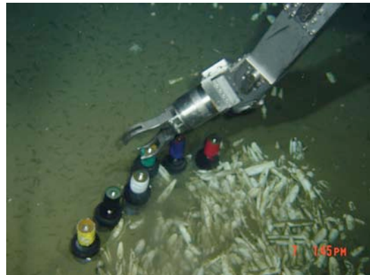
MBAR type core sampling
