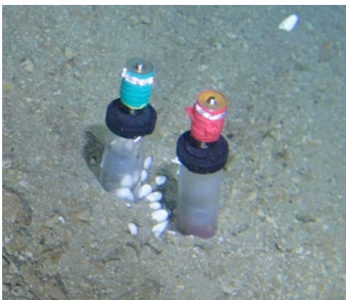
Two MBARI corers. A clam In the right corer was destroyed during the core insertion and red blood oozed out from the clam.
