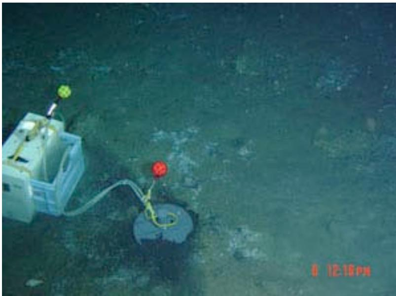
Fig. 7.2-2 Deployment of No. 5 CAT-meter
