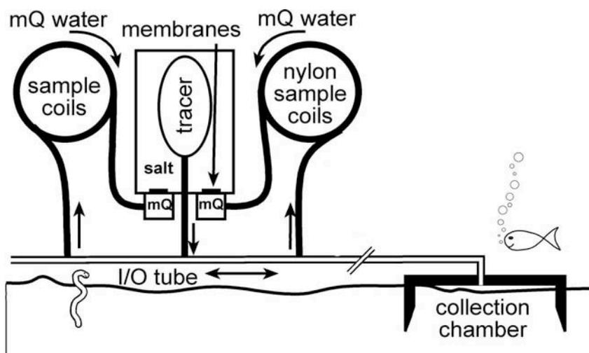
Fig. 5.1-1 Schematic diagram of CAT meter.
