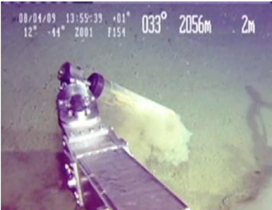
Figure 7.3-11: MBARI push coring (black: C2) was performed for reference outside the spaghetti-like worms in the blight spots area (Point 9). 1:55pm. (from video camera 1)
