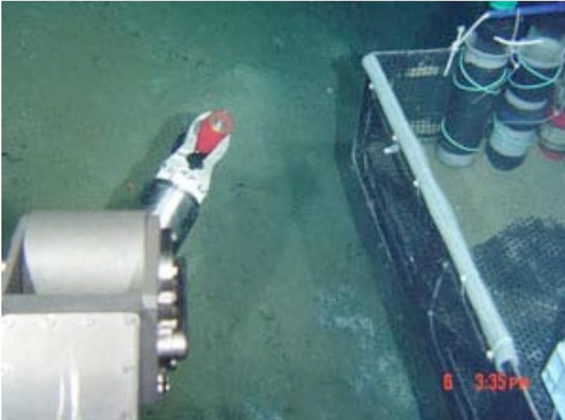
Fig. 7.2-12 Sampling core sediments by MBARI (Red)
