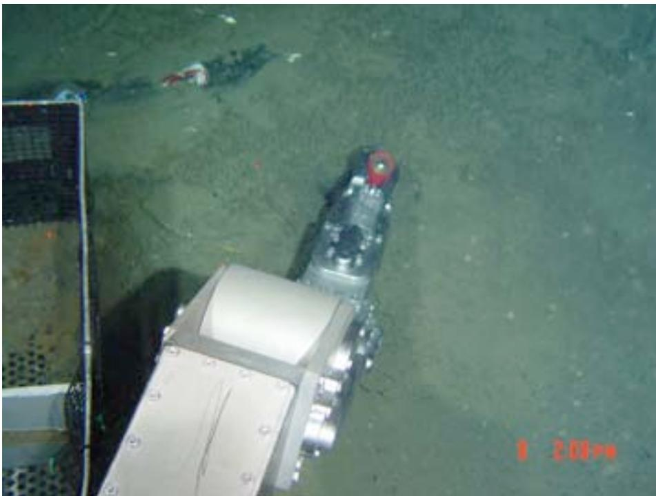
Figure 7.3-13: MBARI push coring (red: C3) was performed on the spaghetti-like worms in the blight spots area. 2:09pm. (Point 11)
