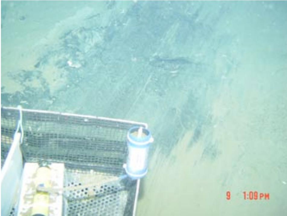
Figure 7.3-8: Scraped mud indicated sulfate black although the normal surface showed brown mud. 1:09pm.
