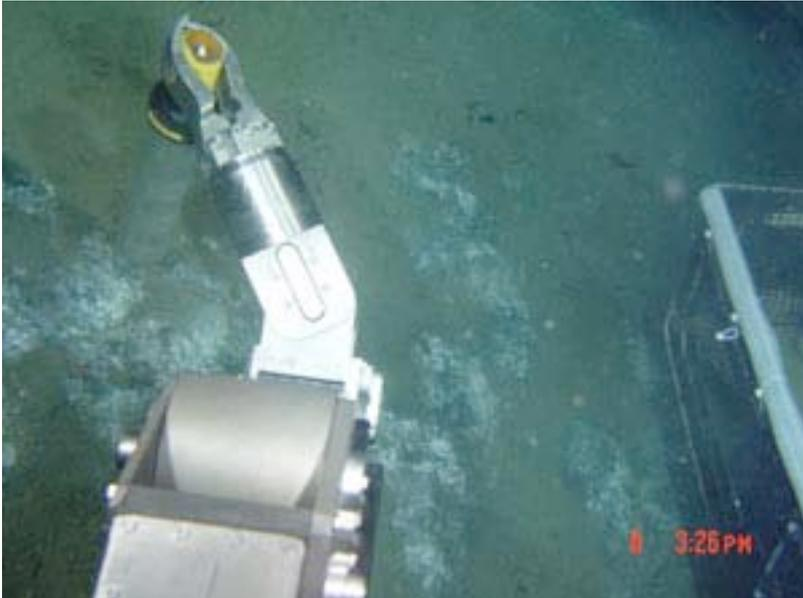
Fig. 7.2-11 Sampling core sediments by MBARI (Yellow)
