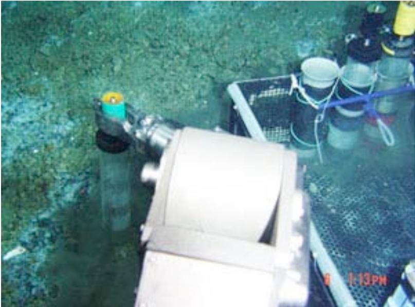
Fig. 7.2-6 Sampling core sediments by MBARI (Green)
