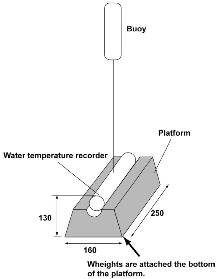
Fig. 5.3-1 Schematic illustration of Bottom-water temperature monitoring system
