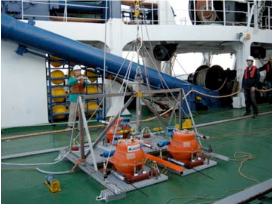
Fig. 5-4-2-2. A simplified ocean-bottom benchmark
