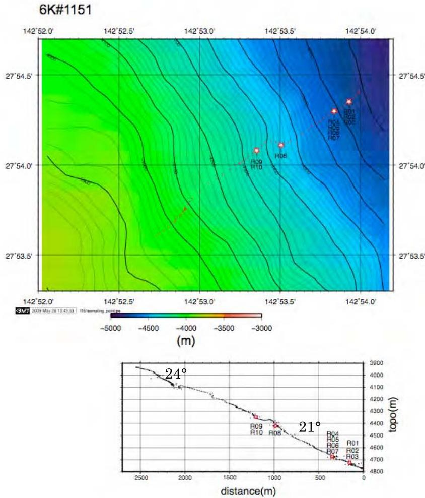
Figure 1 Topographic map and sub track (upper) and topographic section based on depth data of the sub (lower). Average inclination of the slope is shown on the lower figure.
