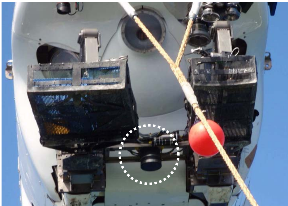
Fig. 3-5 Sub-bottom transducer installed on Shinkai 6500
