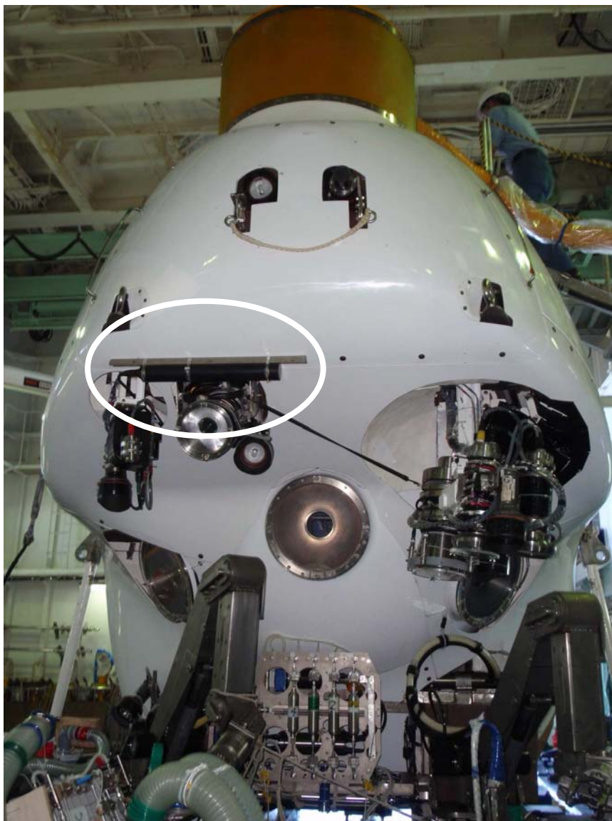
Fig. 3-6 “Shinkai-Miniko” installed on the Shinkai 6500 .
