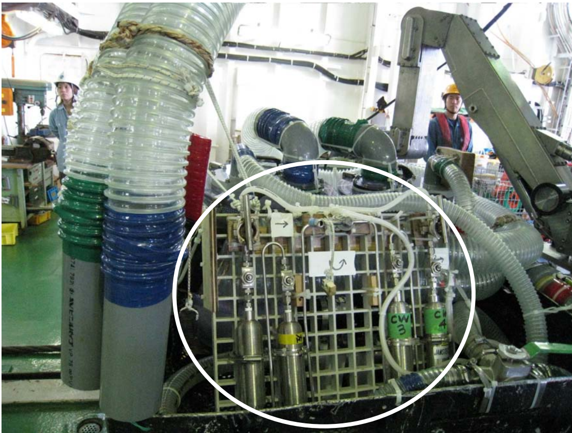
Fig. 3-9 Cheep WHATS sampler installed on Shinkai 6500.
