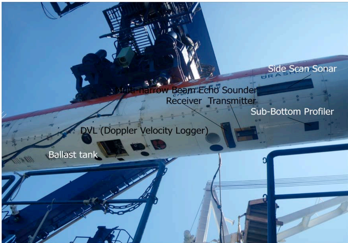
Fig. 4. MBES, SSS, SBP, and other instruments below the Urashima.
