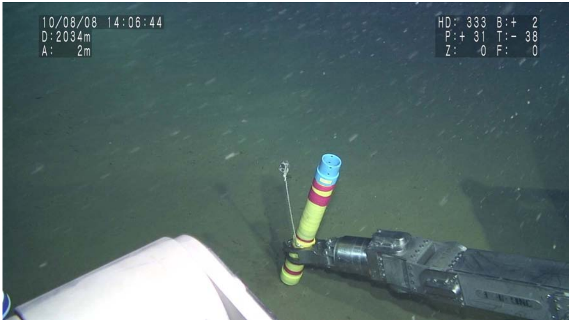
Figure 4.2.2.8: Measurement of heat flow by SAHF at point SAHF3
