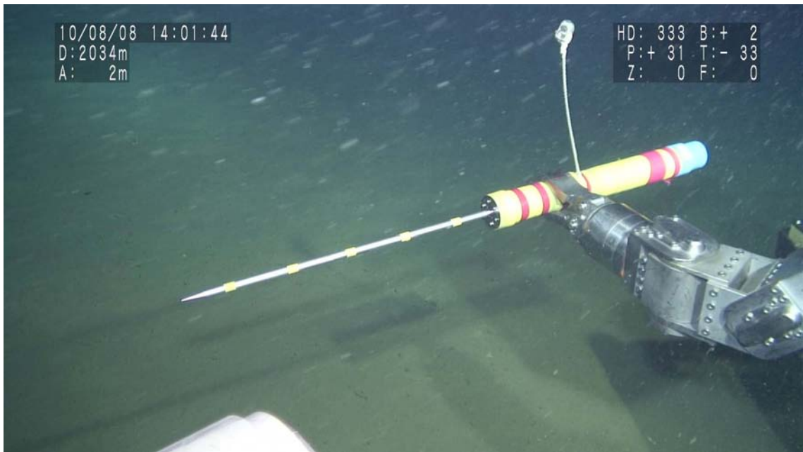
Figure 4.2.2.7: Calibration of SAHF prior to SAHF3 measurement.
