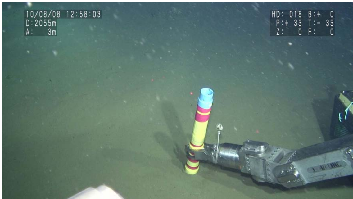
Figure 4.2.2.5: Measurement of heat flow by SAHF at point SAHF1
