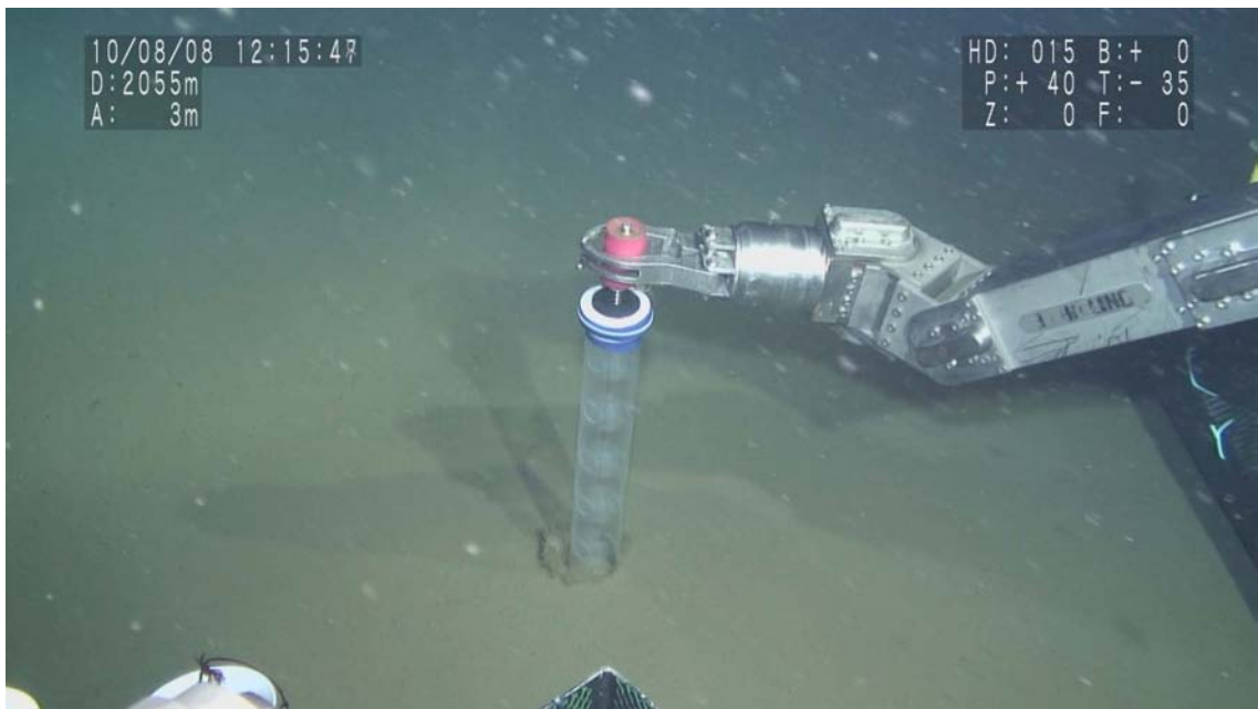
Figure 4.2.2.3: Sampling sediment from the seafloor of east foot where we expected that the mud dike exposes up to surface sediment according to the AUV exploration.
