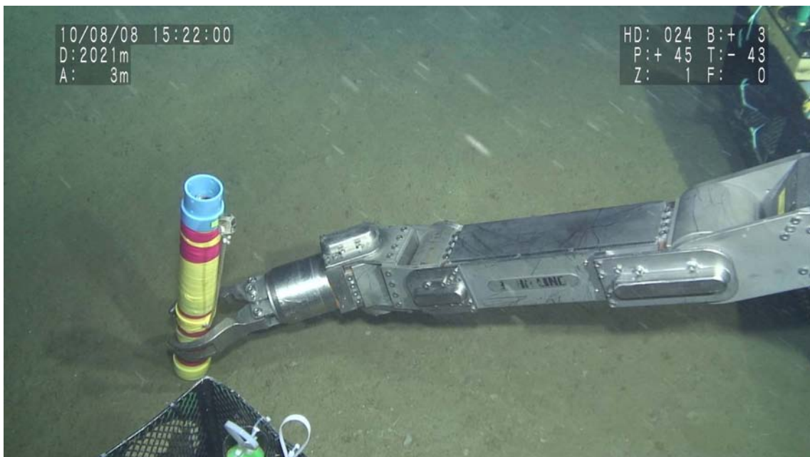
Figure 4.2.2.13: Measurement of heat flow by SAHF at point SAHF5
