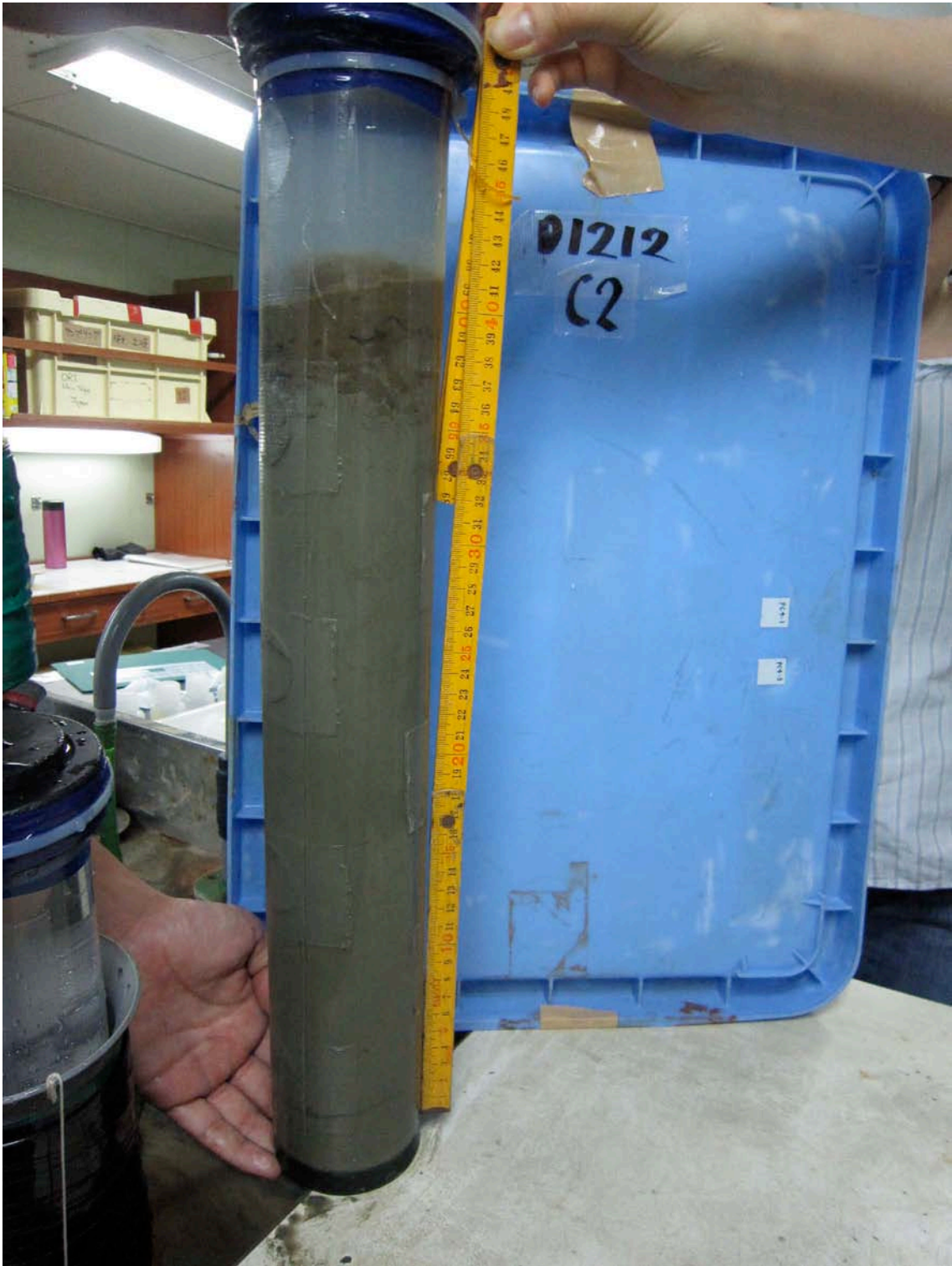
Figure 4.2.2.18: MBARI-type push corer (yellow: C2)
