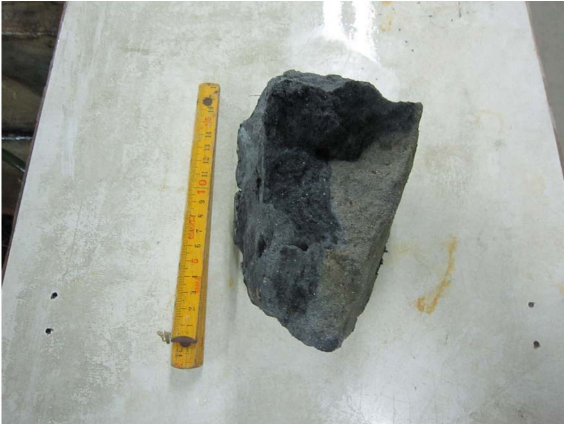
Figure 4.2.1.10 Sandstone blocks with blacky-coated sulfate.
