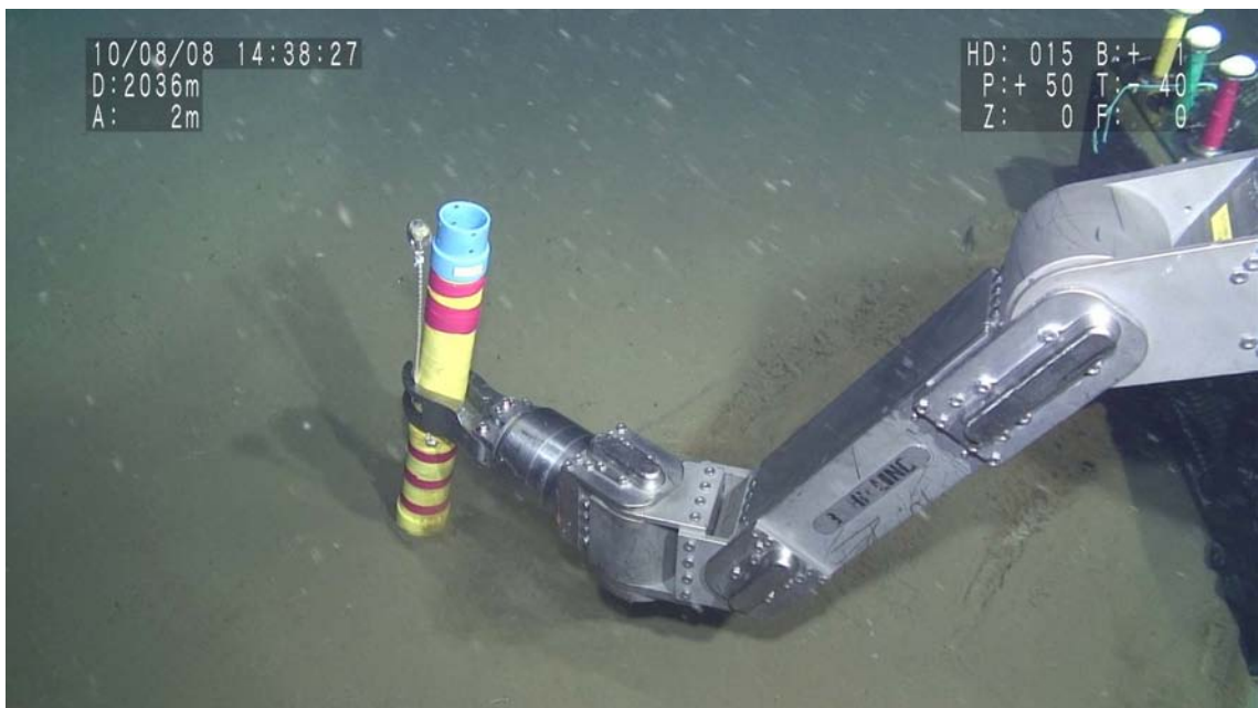
Figure 4.2.2.11: Measurement of heat flow by SAHF at point SAHF4
