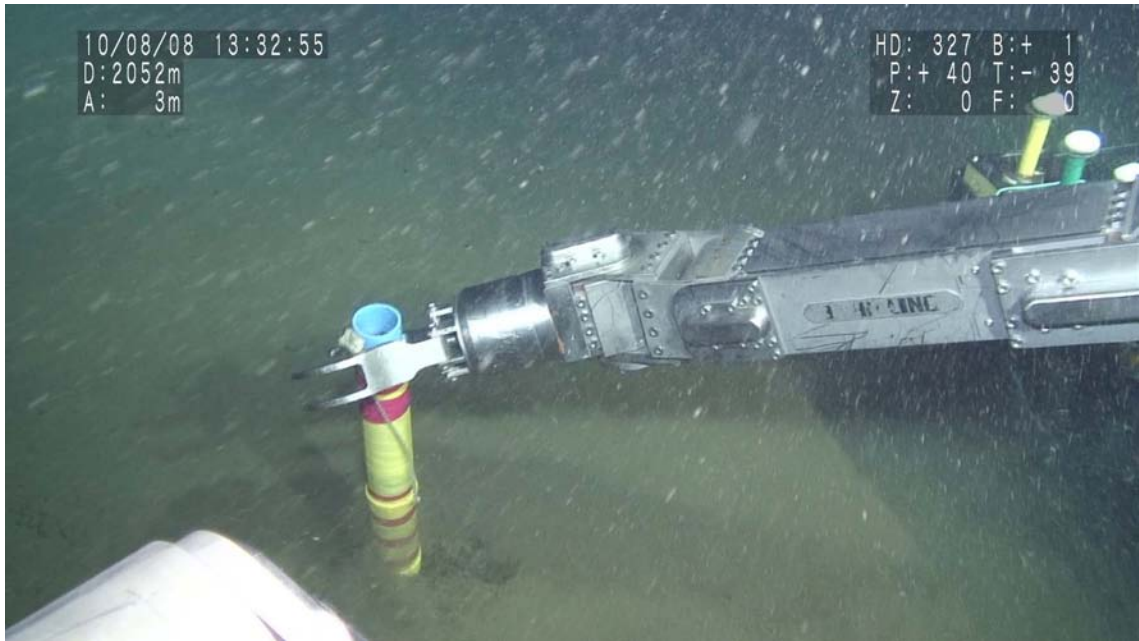
Figure 4.2.2.6: Measurement of heat flow by SAHF at point SAHF2
