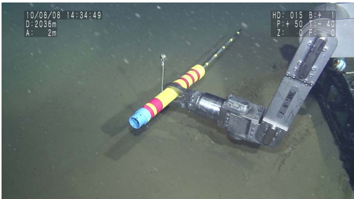
Figure 4.2.2.9: Calibration of SAHF prior to SAHF4 measurement.
