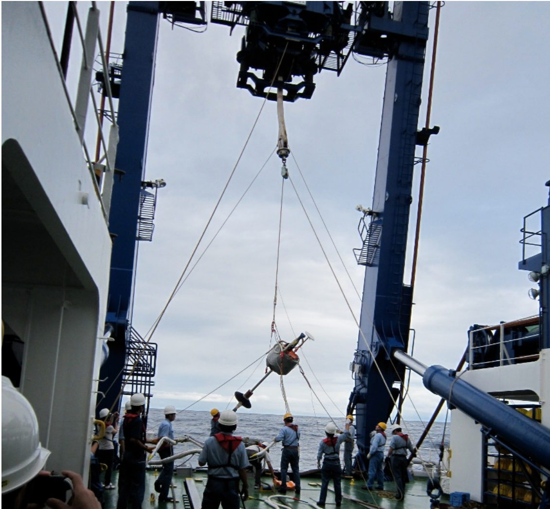
Figure 5.2. Overview of the deployment operation using A-frame.
