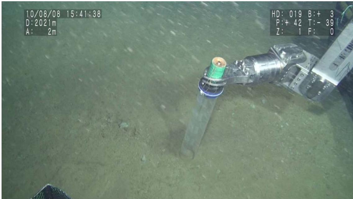
Figure 4.2.2.14: Sampling sediment from the top of the Kumano Knoll No.8 close to SAHF5 after SAHF measurement.
