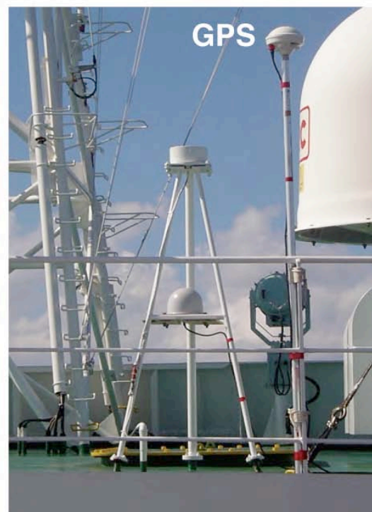
Fig. 4-1 Kobe University type shipboard three-component magnetometer system.
