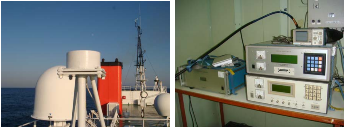
Fig. 6-3-4 The fluxgate magnetometer sensor is mounted on the Nav. Deck (left). The SFG-1212 system is installed in No.1 study room.
