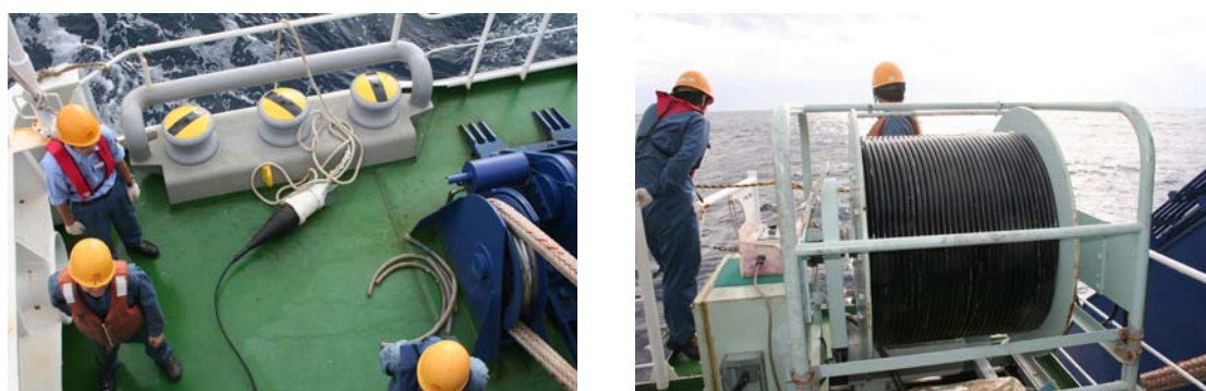
Fig. 6-4-2 A view of the proton magnetometer sensor (left) and tow cable winch (right).
