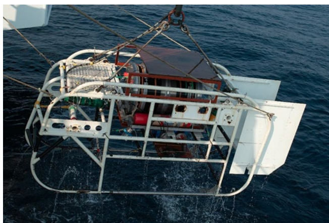
Figure 3.3.1. A snapshot when the deep tow equipped with the FC system is retrieving.
