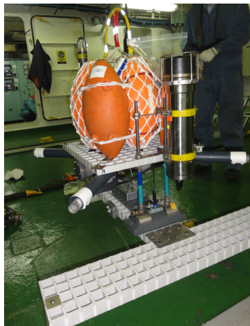
Fig. 5.2.3 Photo of new OBEM system designed to deploy around the rough topographic area.
