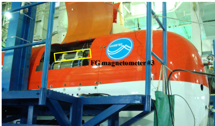
Fig.6.3.1 FG magnetometer #3 installed in forebody payload space.
