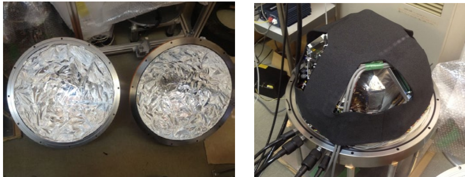
Fig.4 Adiabatic insulation. The spring of S-174 requires constant high temperature, 60.4 °C. We increase adiabatic insulation additionally.
