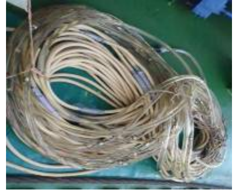
Photo. 4-5-1. Air-gun (left) and single channel hydrophone streamer cable (right)
