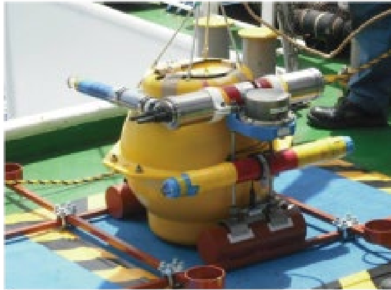
Photo 4-4a. OBM (titanium cylinder) attached horizontally to glass sphere OBS.
