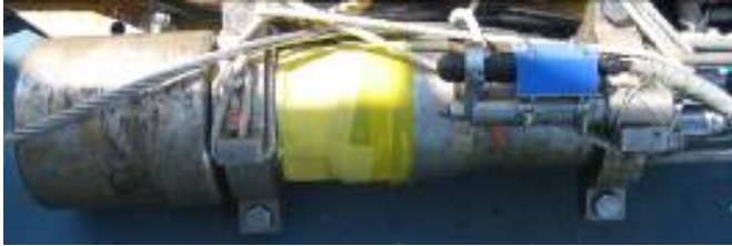
Photo. 4-5-1. Air-gun (left) and single channel hydrophone streamer cable (right)
