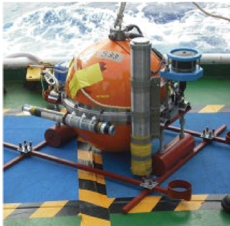
Photo 4-4b. OBM (titanium cylinder) attached vertically to titanium sphere OBS.
