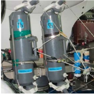
Bag water sampler (400 \times 200 \times 270mm, weight-in-air: ca 4kg)
