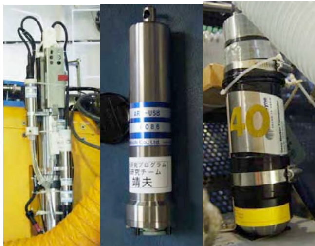
Fig. 5. The CTD-DO (left), DO sensor (center), and ROV-homer (right).
