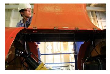
Figure 4 Hydrophone mounted on the Urashima vehicle
