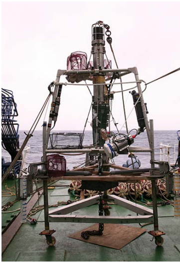
Figure 3-2: Deep-sea camera system. Figure 3-3: HDTV camera equipment used for the video recording.
