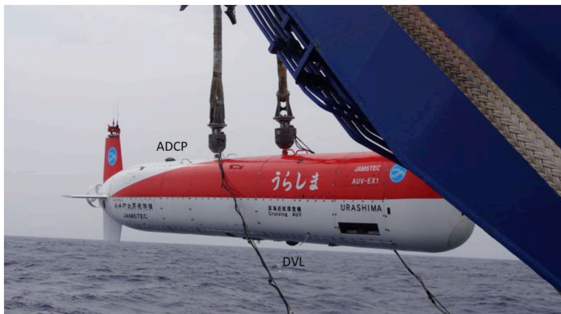
Fig.4.4 The ADCP and DVL mounted on the Urashima.
