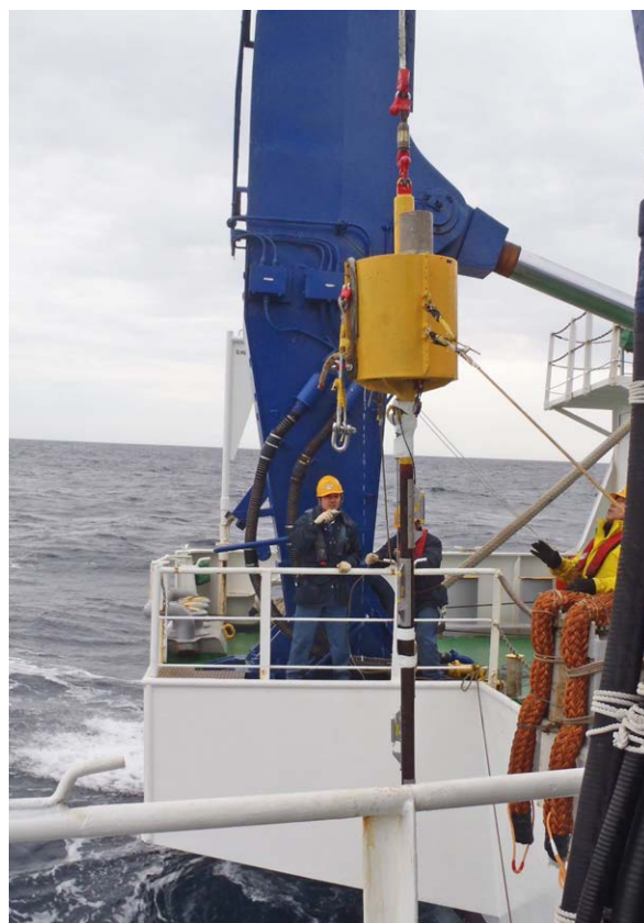
Figure 3.5-1. Heat flow measurement operation.
