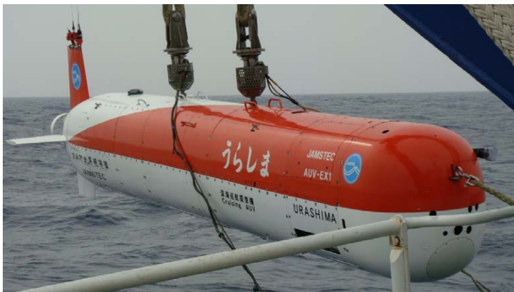
Fig.4.1 Overall feature of a cruising AUV Urashima.
