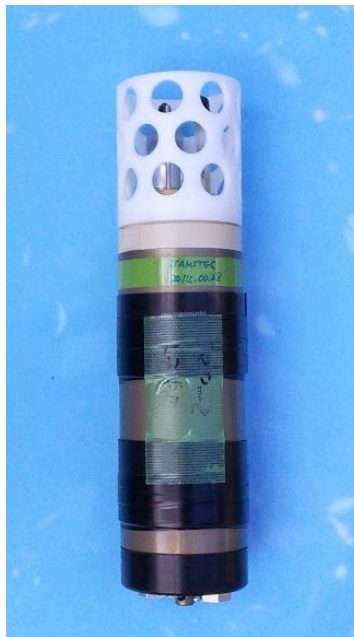
Arrangements of the pH meter installed in Urashima .
