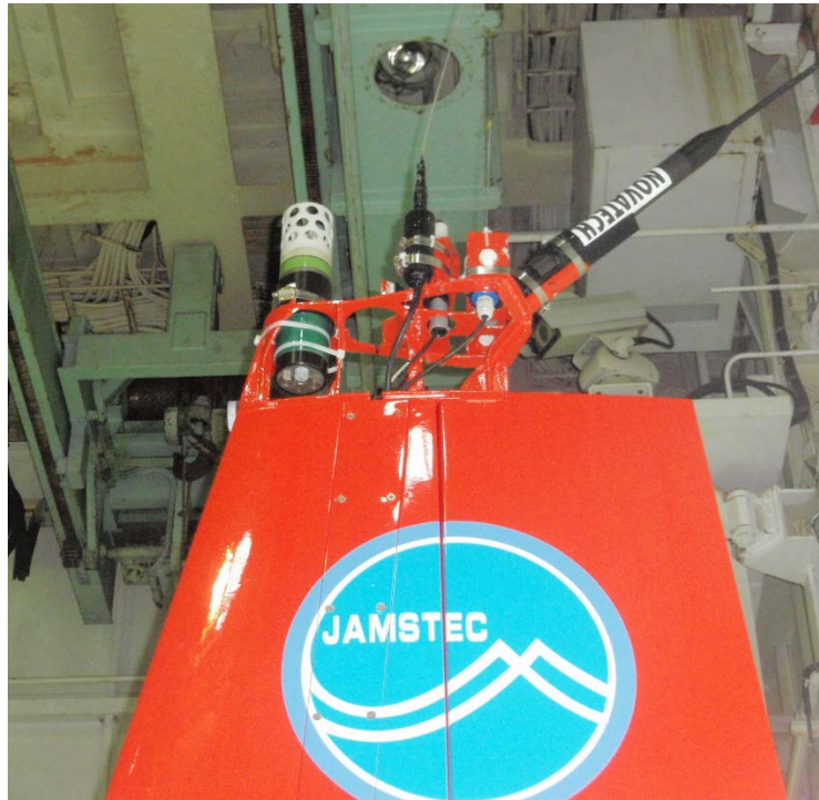
Arrangements of the pH meter installed in Urashima .
