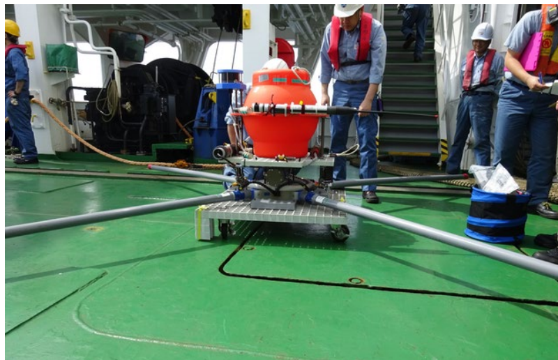
Figure 3.4-3. Photo of a pop-up type OBE system.
