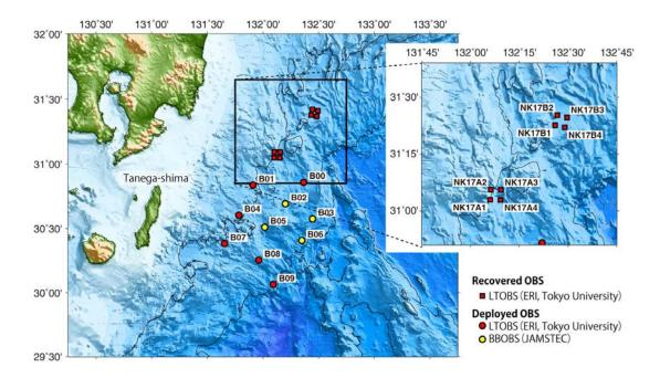
Figure 1. Map of study area. Red Squares represent recovered Long-Term OBSs (LTOBS). Red circles are the deployed LTOBSs, and yellow circles mean the deployed broadband OBSs (BBOBS). A Pressure-Temperature logger (RBR TD 10000) is fixed on the rim of the BBOBS.
