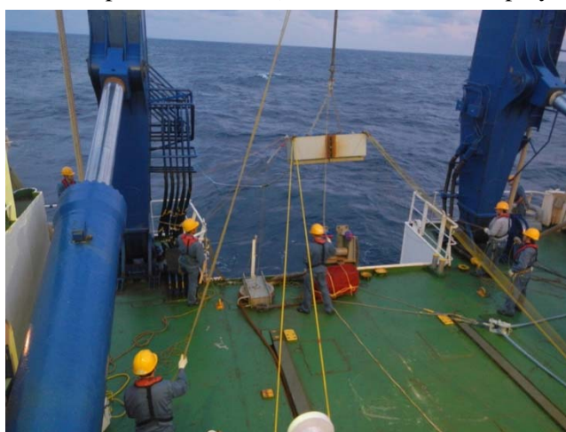
Figure 7: Block anchors deployed through the A-frame.
