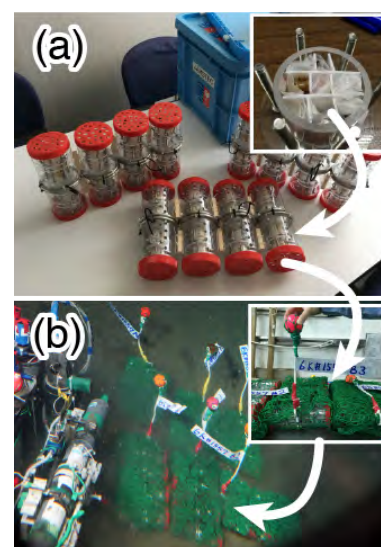
Fig. 1. (a) sample chamber and (b) deposited sample chamber on the deep-sea floor.
