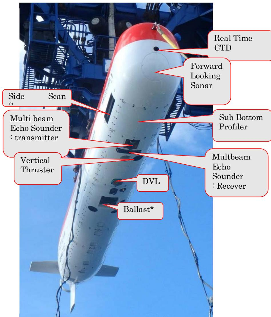
**Figure 4-1: Sensors and instruments on Urashima. \*A 125kg ballast assembly is lathed this position, and released at the end of the survey. This photograph was taken at the AUV retrieval.**
