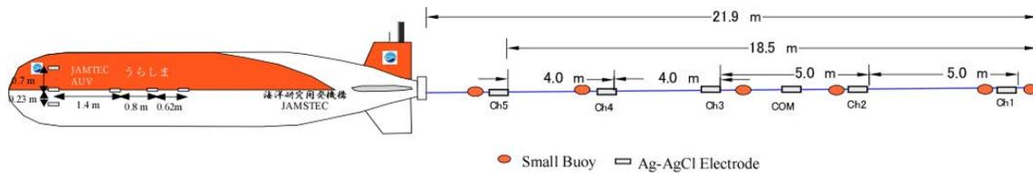
**Figure 4-2 Electrode's configuration on the AUV URASHIMA**
