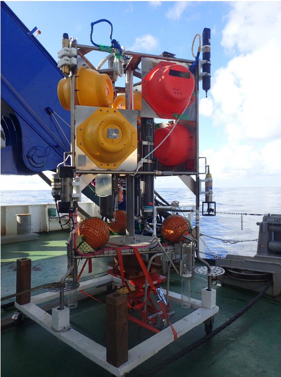
Fig. 3.3.2. Niskin bottles on lander system
