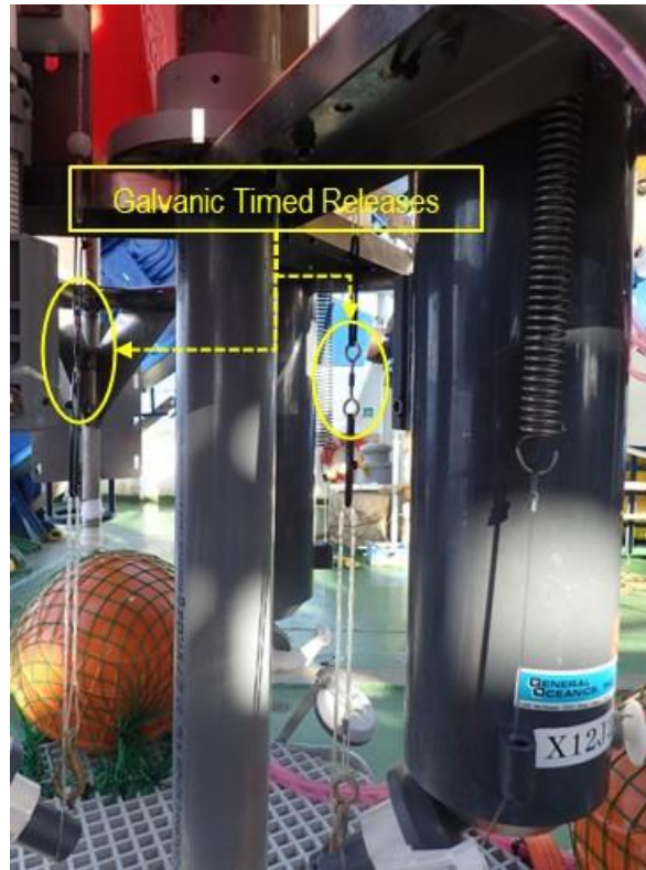
Fig. 3.5.12. Galvanic Timed Release set in a Niskin water sample.
