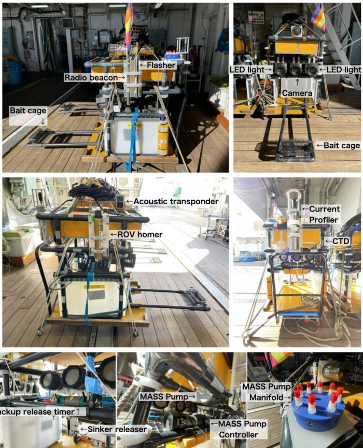
Fig. 3.4.1. Baited camera and equipment
