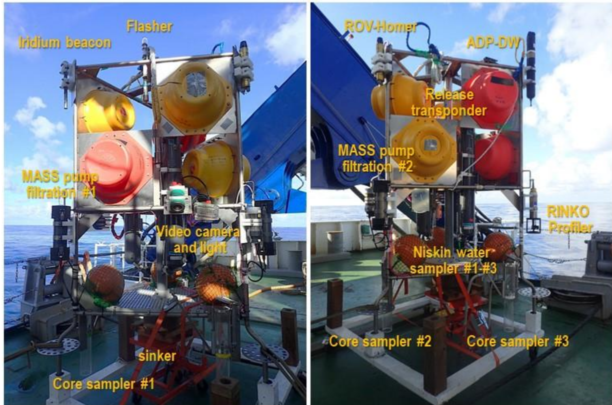
Fig. 3.5.2. Configuration of the Lander System
