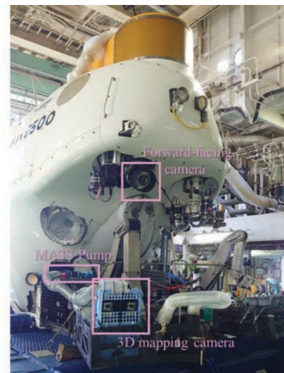
Fig. 3.2-1 Cameras and pump on the Shinkai.
