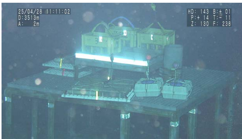
Fig.3 Photo of the condition of all specimens on the platform before the recovery operation.
