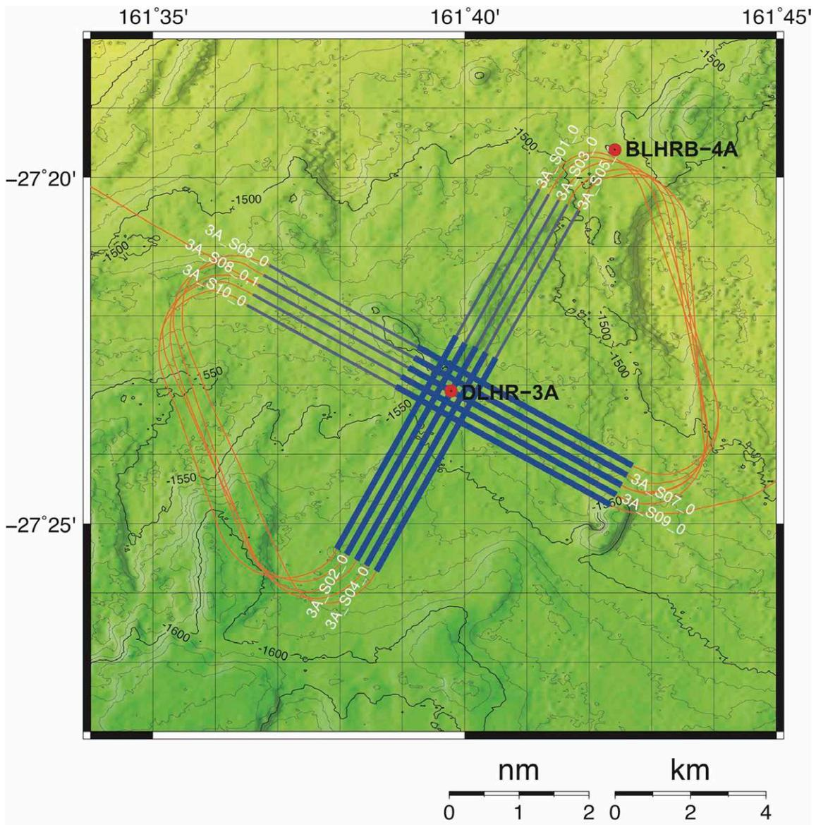
Figure 11. HR-MCS survey lines in the DLHR-3A area. Blue thin and thick lines indicate regions of air gun shooting with partial volume and full volume, respectively. R/V Kairei's track during the OBS-MCS survey is shown by orange line.
