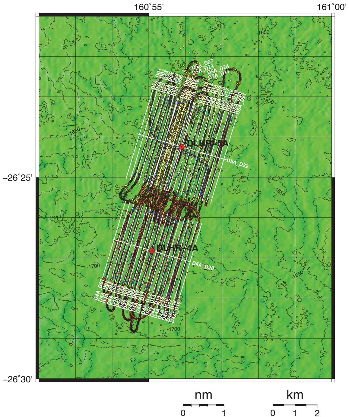
Figure 6. 6KSDT sonar survey planned lines and way points. White thick lines are planned survey lines. Yellow and orange dots are way points of the towfish during Leg 1 and Leg 2-2, respectively, as positioned by the shipboard Acoustic Navigation System (ANS). Blue dots are end points of surveyed lines positioned by ANS.
