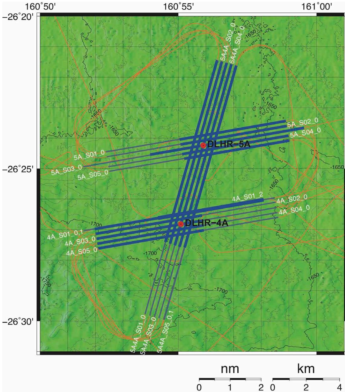
Figure 10. HR-MCS survey lines in the DLHR-5A/4A area. Blue thin and thick lines indicate regions of air gun shooting with partial volume and full volume, respectively. R/V Kairei's track during the OBS-MCS survey is shown by the orange line.
