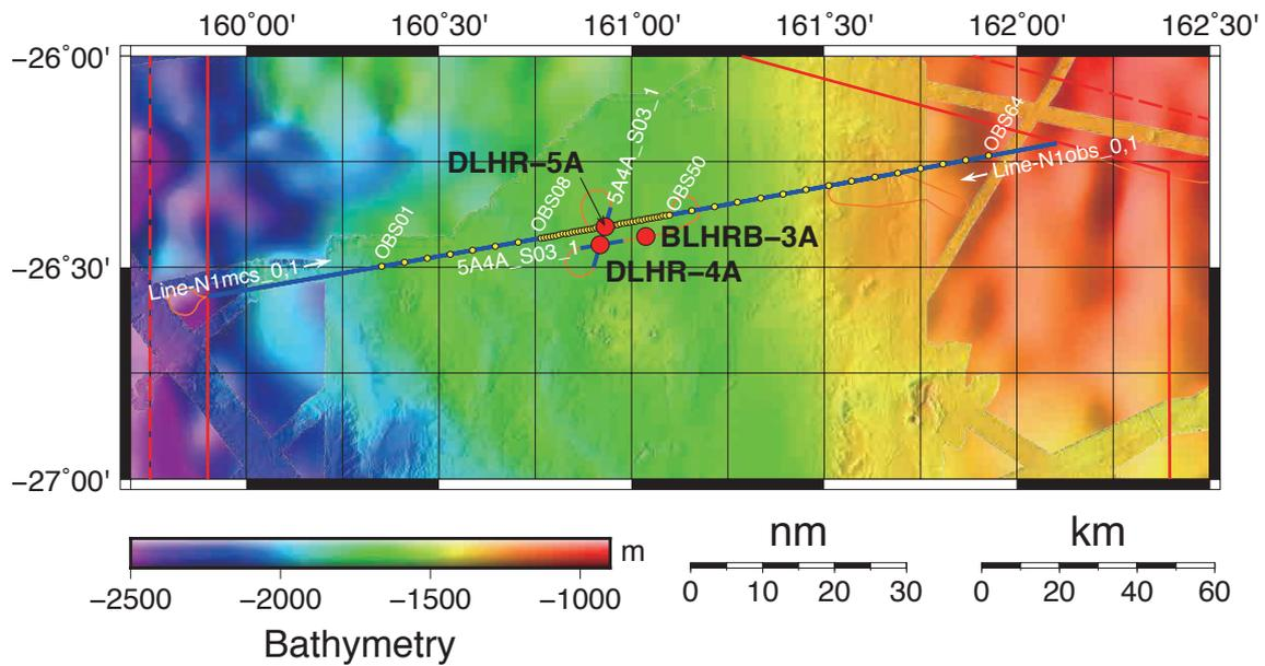
Figure 12. OBS-MCS survey lines (blue lines) and deployed OBS positions (yellow dots). R/V Kairei's track during the OBS-MCS survey is shown by orange line.
