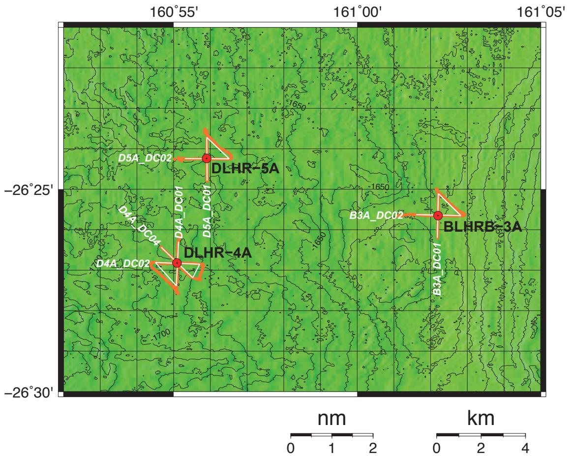
Figure 7. 6KSDT camera survey way points. White thick lines are planned survey lines. Orange dots are way points of the towfish positioned by phins DVL.
