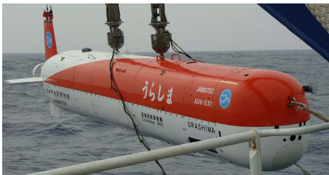
Fig.2.1 Overall feature of a cruising AUV Urashima.
