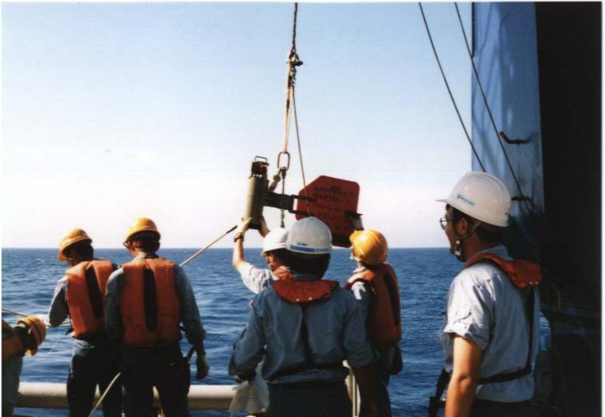
Deployment of current meters of mooring buoy
