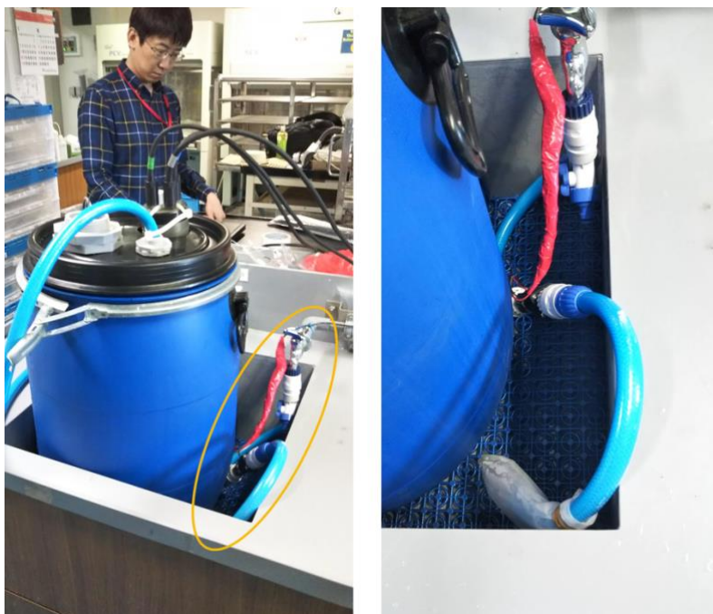
Fig. 2. The microplastic sampler installed to the outlet of the onboard seawater pump of D/V CHIKYU.
