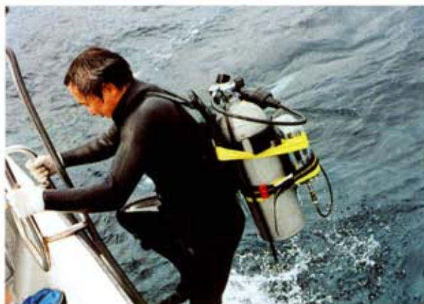
Photo 2 The equipment that measures and records the actual respiratory condition of the research diver (It can be seen on the air cylinder on the diver's back.)
