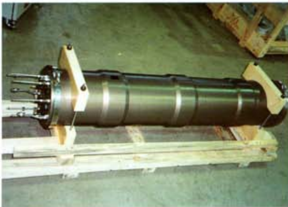
fig.6 Under real sea area test Fuel cell
