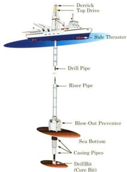
fig.1 Deep-sea drilling vessel system
