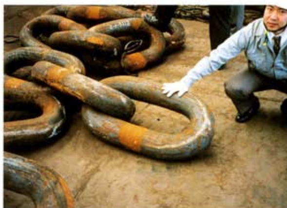
Fig. 3 Mooring chain link
