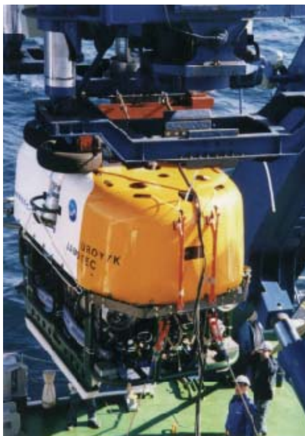
Photo 10 Scene of UROV7K hoisted up by an A-frame crane
