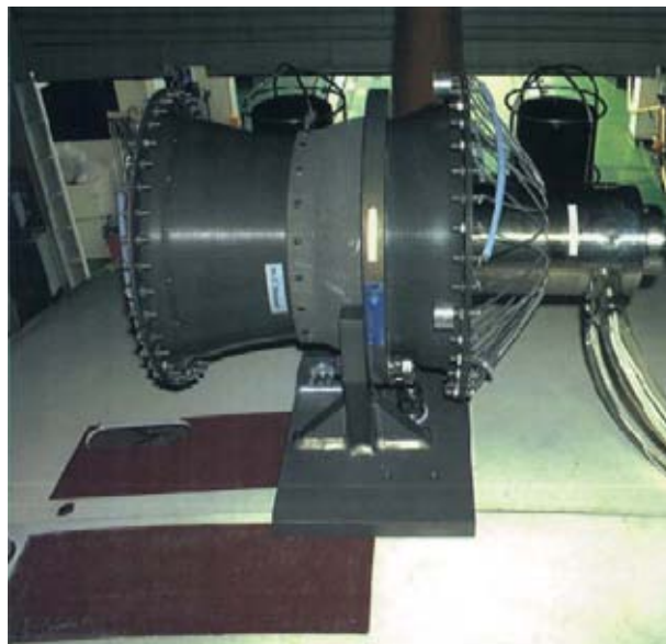
Photo 9 Thruster mounting onto the top of "Shinkai 6500"
