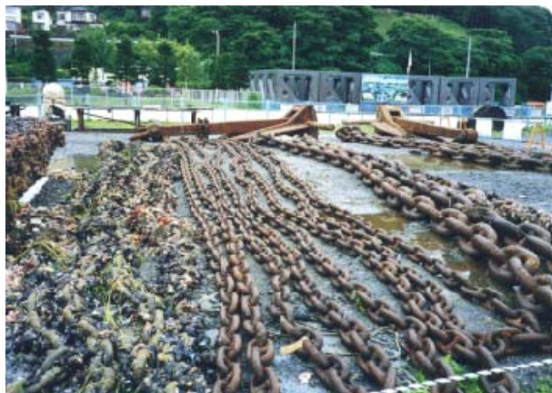
Photo 3 Mooring system collected for on-land inspection
