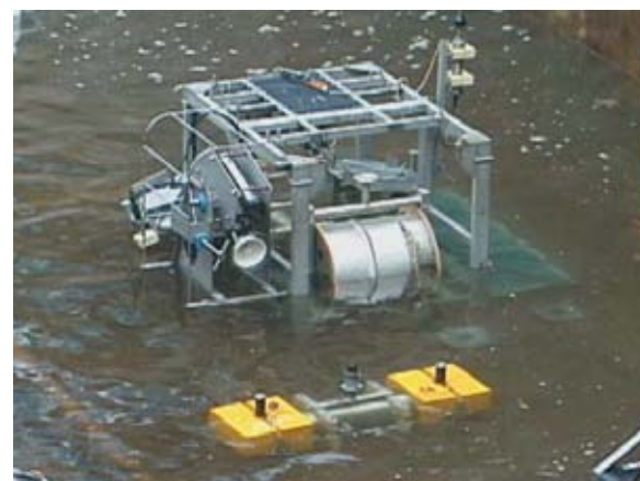
Photo 7 Multi-sensor package unit and seismogram during the on-land trial test.
