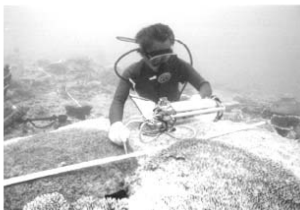
Photo 1 Measurement of photosynthetic activity using fluorescence meter
