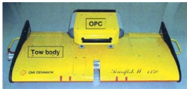
Photo 8 Optical plankton counter (OPC) mounted on the tow body.
