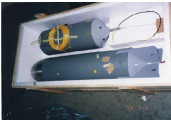
Photo 7 Exterior view of optical fiber spooler used in descent test
