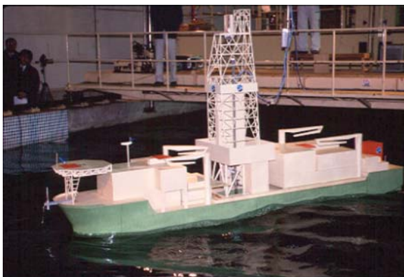
Fig. 2 Test on the Dynamic Positioning System, Control of Riser Inclination
