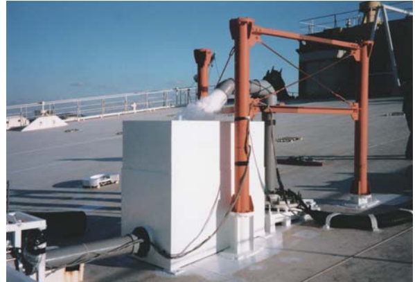
Photo 2 Experiment of seawater drawing by airlift pump
