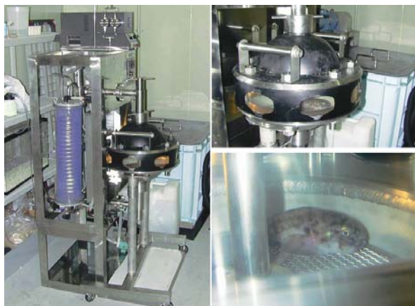
Fig.13 Pressure maintenance-type fish breeding aquarium and Ebinaia brephocephala under pressurization.
