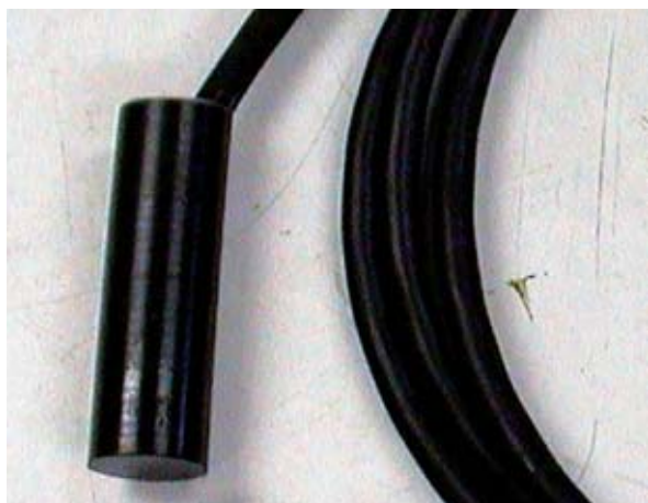
Fig. 2 High frequency transducer (80 ~ 120kHz bandwidth)
