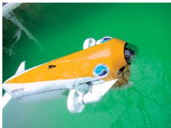
Fig.17 Pool testing of the AUV-ROV hybrid submersible
