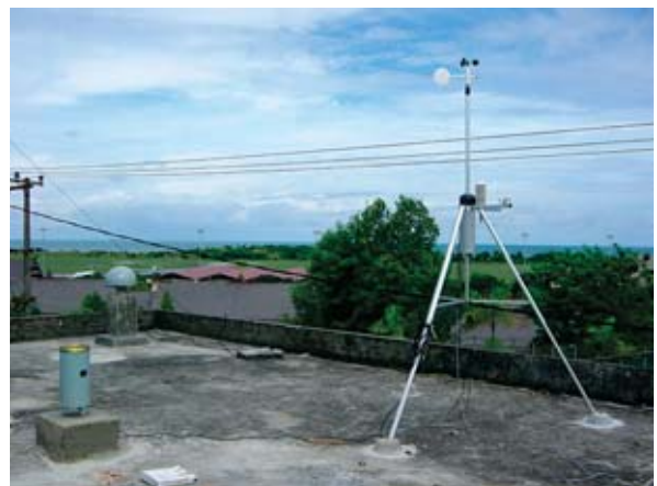
Fig.22 GPS receiver and automatic weather station at Balikpapan, Indonesia.
