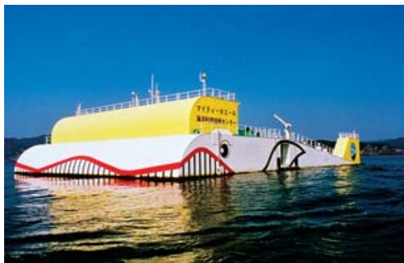
Fig. 7 Offshore floating wave power device the "Mighty Whale"
