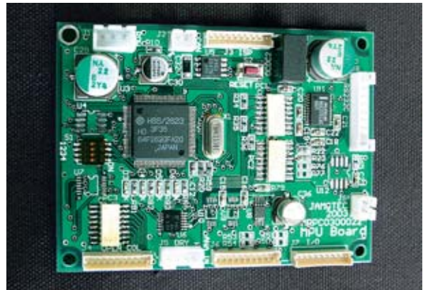
Fig.13 Hardware prototype for control platform
