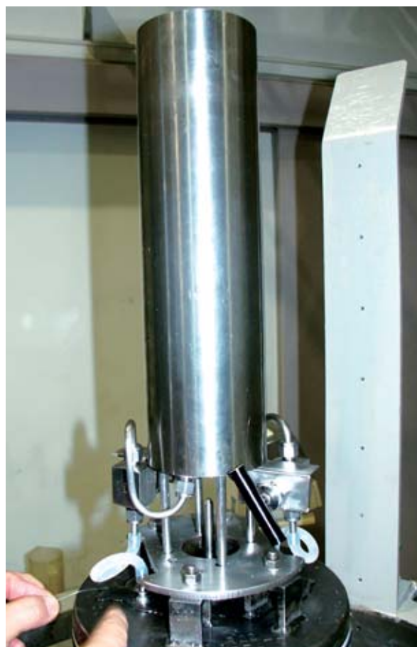
Fig.18 Piston type internal titanium tank
