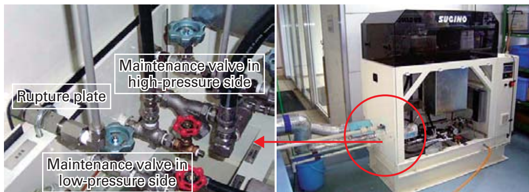
Fig. 3 Hyperbaric experiment water tank, Pressurization equipment
