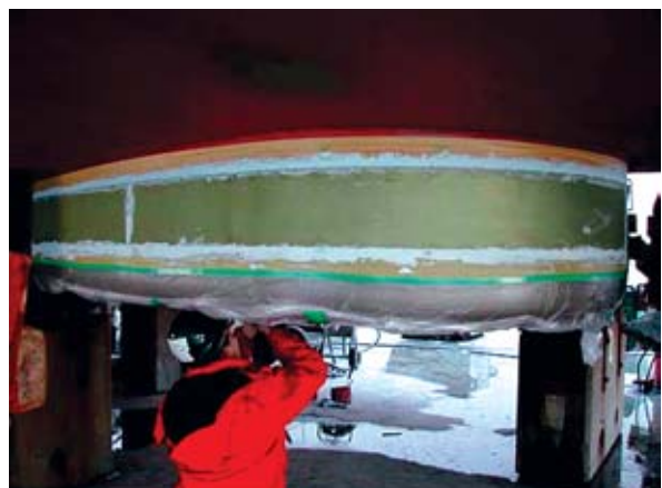
Fig. 4 Transducer dome of multi-narrow-beam echo sounder
