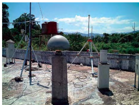
Fig. 8 Observational system in Kototabang, west Sumatra, Indonesia. Automatic climate observational equipment (back left), GPS antenna (front), rawinsonde receiver (back right).
