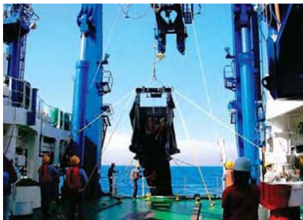
Photo 1 The multi-net system, IONESS.
