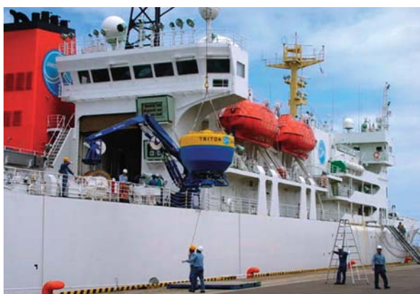
Fig. 9 Loading work of TRITON Buoy after maintenance to R/V MIRAI at Mutsu Institute for Oceanography.
