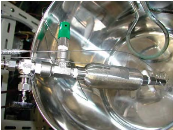
Fig.18 Oxygen gas storage test container.
