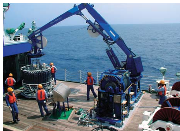
Fig. 5 Observation work by CTD on R/V MIRAI .
