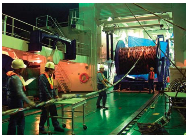
Fig. 4 Streamer cable installation work on R/V KAIREI .
