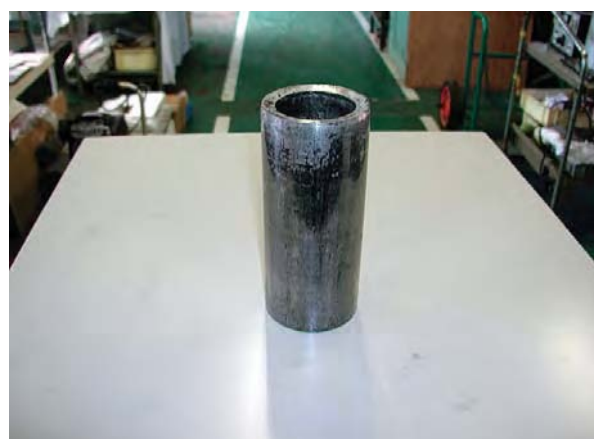
Fig. 8 Pressure-tight container made of magnesium alloy.
