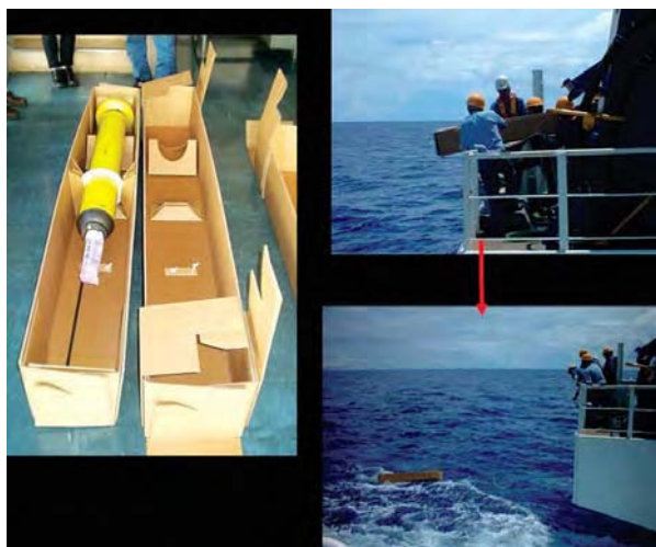
Fig. 3 Launching apparatus to deploy Argo floats from a cruising vessel.
