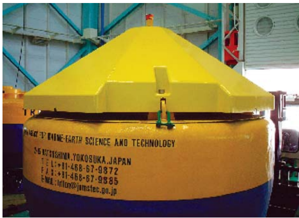
Fig.26 Deck Cover for preventing a theft from getting on the buoy.
