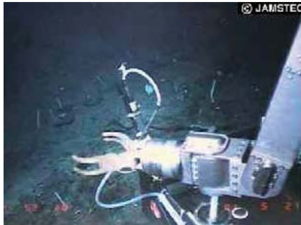
Fig.10 Example of demodulated picture (320 × 225 pixels)(transmission time 1.2 seconds) No error.
