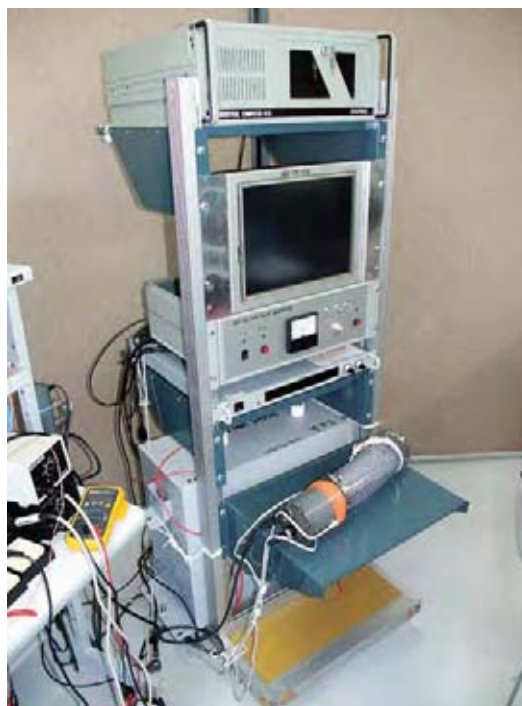
Fig.15 Electromagnetic pulse generator and receiving antenna.
