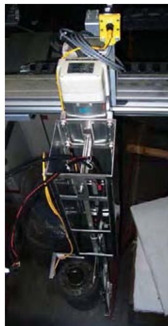
Fig.17 Oscillating device for water tank test.
