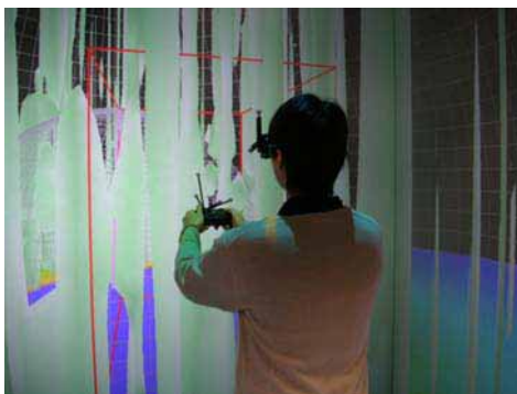
Fig.7 Interactive data analysis of geodynamo simulation with VFIVE in the CAVE's virtual space. It is possible to visualize large-scale data set of the size of 17 GB by ROI extraction function.
