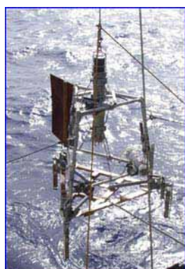
Fig. 4 11,000-m free-fall type camera bottom sampling system
