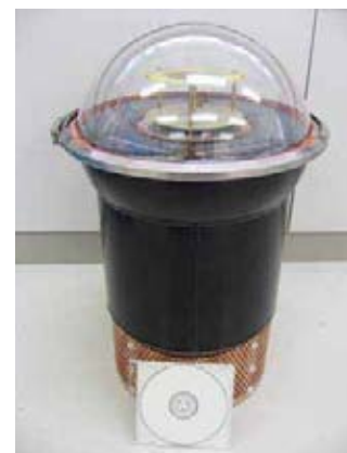
Fig. 11 New float equipped with a solar panel
