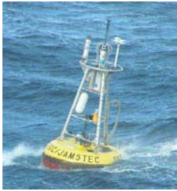
Fig. 4 Sea surface mooring buoy (Height: 5 m from sea surface, Weight in air: 0.85 ton) at the sea surface flux observation site.
