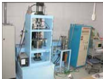
Photo Fluid control-type medium-to-high speed friction tester capable of reproducing the water content, temperature, and pressure conditions of faults more realistically.
