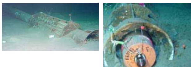
Fig.3 ACORK head observed during the KY07-18 cruise. (Left) Before installing the seal more than half of ACORK mouth is buried beneath the sediment. (Right) Hydrologic seal was installed.
